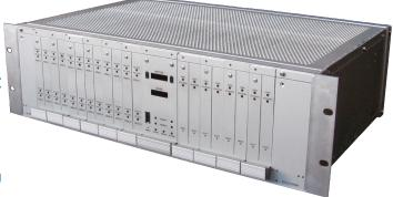
Axle Counter BROS is used to control occupancy of the railway sections. The device is placed into a standard 19-inch 3U height rack and it is mounted inside the relay room of the railway station, automatic block system, or level crossing.
